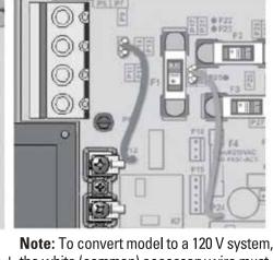
BROWN wire must be correctly connected the white (common) accessory wire must be moved. See wiring diagram for details.
